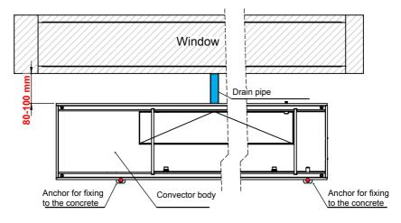
Scheme III. - Connecting to the heating system
